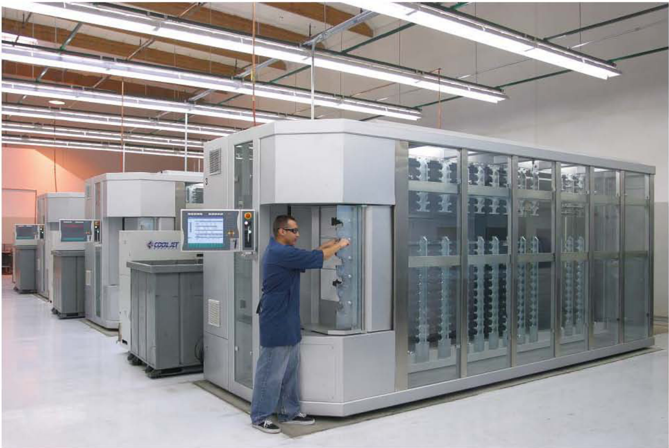
Cell leader Alfonso Banuelos adds tools to the 494-tool magazine on the company's new Toyota FMS. The system has 44 pallets serving 3 Toyota FH450S III 4-axis horizontal machining centers purchased from Selway Machine Tool Company.
